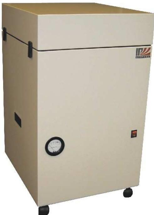
The F1800 series is designed for laser and solder fume removal. Our proprietary fan design ensures a strong suction force and high airflow rates. For low operating costs the unit features heavy-duty pre-filtration and large main-filters. A differential pressure gauge indicates the status of the particulate filter. An optional lid allows the connection of 2", 2.5" and 4" diameter hoses.
